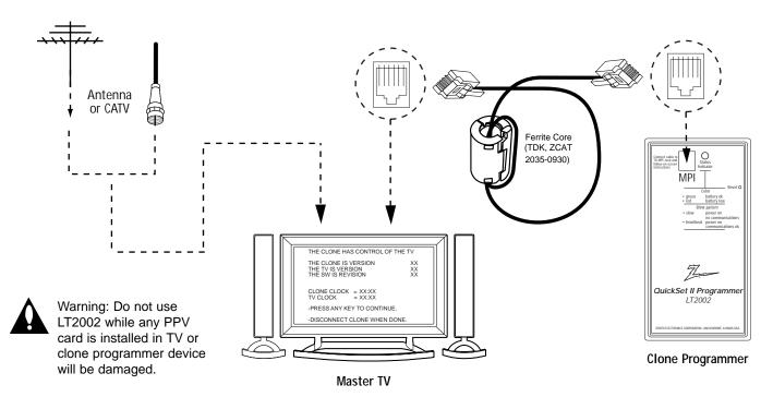
Connections for the LT2002 Clone Programmer to Learn the TV Master TV Setup
